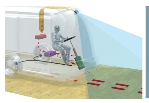
A camera located on the front of the vehicle reads the route; it analyses the divergence between the markings on the ground and the vehicle's position. An interface based on using the steering wheel helps the driver narrow this divergence.
